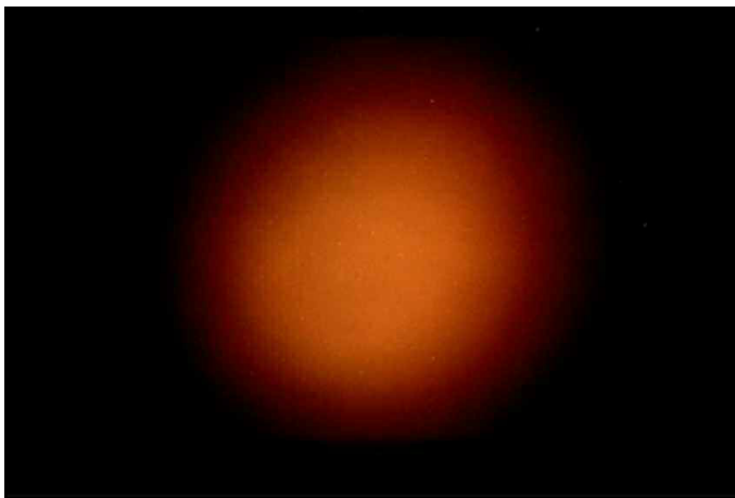
Fig. 3 A stacked set of images, taken in the same sky location as Fig. 1, but with a small slew performed between each image. The stars on sequential images do not overlay; however, the sky-glow is consistent. Thus, a sigma clip will effectively eliminate all stars while retaining properties of the sky-glow (which also includes the characteristics of vignette for the optical system).
